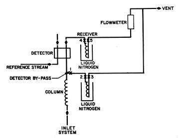
Figure 3. Column, detector, and detector bypass
