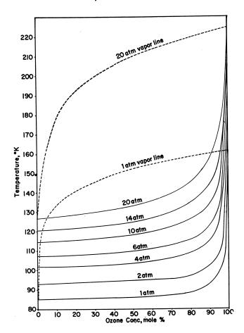
Figure 2. Vapor-liquid equilibrium diagram of ozone-fluorine system
