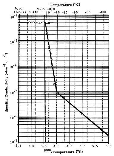
Figure 5. Conductivity of bromine trifluoride as a function of temperature
