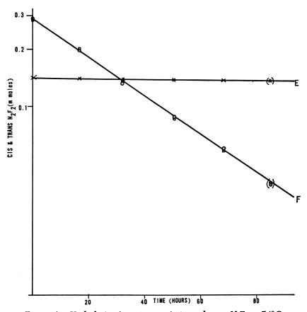
Figure 4. Hydrolysis of a mixture of cis- and trans-N<sub>2</sub>F<sub>2</sub> at 74°C.
