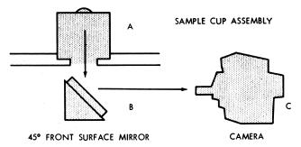
Figure 7. Front surface mirror arrangement; arrows indicate light path. (A) sample cup assembly, (B) 45° front surface mirror, (C) camera.
