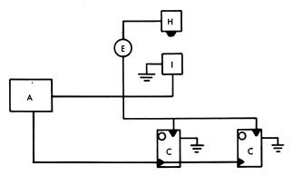
Figure 4. Block diagram of instrumentation on dropweight apparatus. A = Wheatstone bridge; E = 22volt battery; H = drop-weight hammer; I = assembly containing sample cup and pressure gage; C = oscilloscopes
