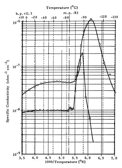
Figure 3. Conductivity of chlorine trifluoride as a function of temperature.  $\Delta$ —before low temperature fractionation; 0—after low temperature fractionation
