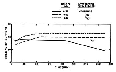
Figure 7. Interrupted electrolysis. KF = 1 mole %, volts = 6.0-6.1, temperature =  $10^{\circ}-14^{\circ}C$ .
