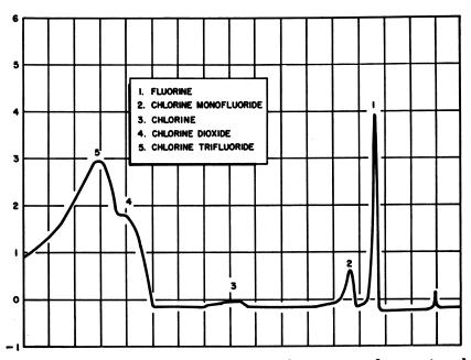
Figure 7. Chromatogram of chlorine trifluoride reaction with unpassivated inlet
