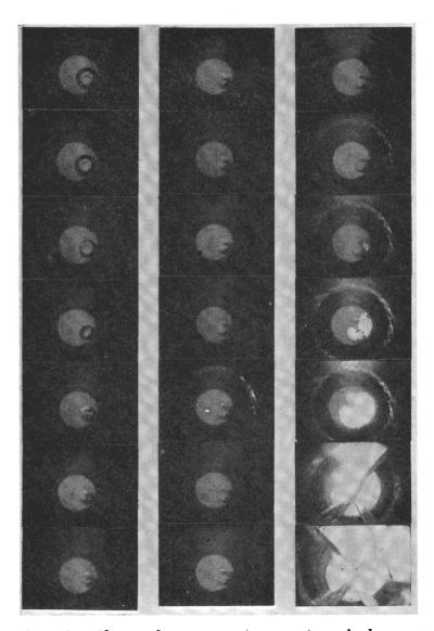
Figure 12. Photographic sequence of compression and subsequent explosion owing to impact momentum and energy well above 50% probability of explosion; interframe time-55.6µsec. Sequence is top to bottom, left to right
