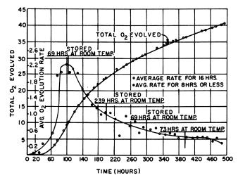
Figure 2. Oxygen evolution of NO<sub>2</sub>ClO<sub>2</sub> at 65°C.
