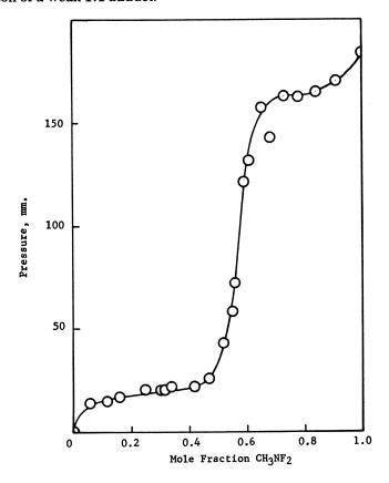
Figure 2. The CH<sub>3</sub>NF<sub>2</sub>-SO<sub>3</sub> system at -45.2°C.
