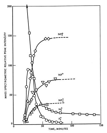
Figure 4. NF: irradiation product analysis. Time vs. peak intensity at 77°K.
