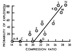
Figure 10. Probability of explosion vs. compression ratio for nitroglycerin impacted from a height of 1 cm. with varying weights using precompression to various initial pressures
