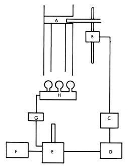
Figure 6. Block diagram of apparatus for photographic studies. (A) drop-weight tester, (B) solenoid, (C) triggering unit, (D) delay unit, (E) camera, (F) counter, (G) 22.5-volt battery, (H) flash unit.
