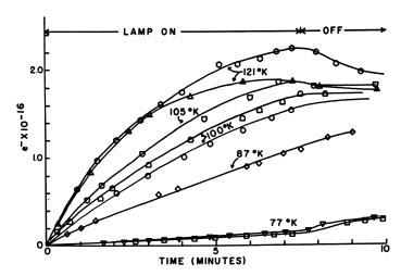
Figure 5. Variation in paramagnetic resonance of photolyzed OF2 at selected temperatures
