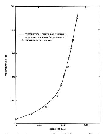
Figure 5. Temperature profile of a hydrazine perchlorate deflagration wave. Strand composition: 94.5% hydrazine perchlorate, 5% Delrin, 0.5% magnesium oxide; density: 1.85 grams/cc.; pressure: 0.5 atm.; deflagration rate: 0.09 cm./sec.
