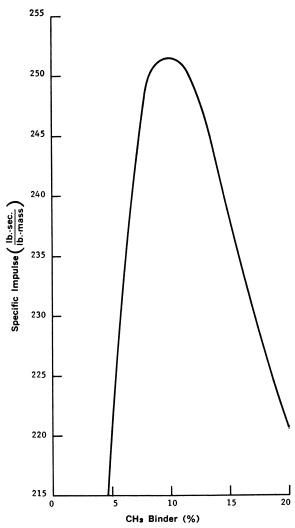
Figure 1. I., vs. percent binder for a  $+CH_2+_x/AP$  propellant
