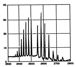
Figure 6. Near infrared spectrum of hydrogen fluoride in ClF:
