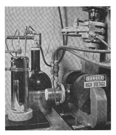
Figure 2. Apparatus for irradiation with high energy photons
