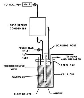
Figure 1. HF electrolysis cell
