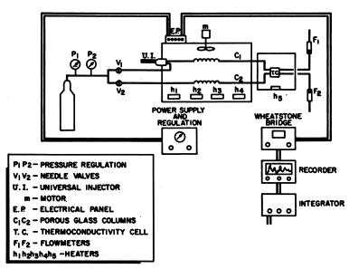
Figure 2. Gas chromatograph for analysis of NTO
