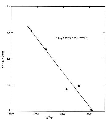
Figure 1. Rate of vaporization of hydrazine perchlorate
