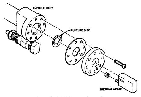
Figure 2. Exploded view of ampoule
