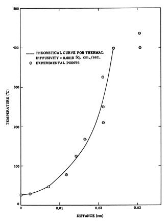
Figure 6. Temperature profile of a hydrazine perchlorate deflagration wave. Strand composition: 94.5% hydrazine perchlorate, 5% Delrin, 0.5% magnesium oxide; density: 1.24 grams/cc.; pressure: 1 atm.; deflagration rate: 0.3 cm./sec.
