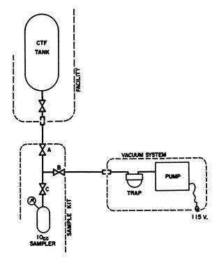
Figure 4. ClF. sampling schematic
