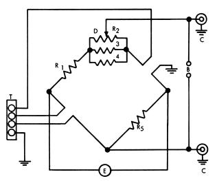
Figure 3. Bridge circuit.  $R_1 = R_5 = 120$  ohms;  $R_2 = 100$  ohms (10 turns);  $R_3 = R_4 = 10$  ohms; B = 2 zero balance checkpoint to galvanometer/potentiometer; C = signal output to oscilloscope; D = balance control; E = 6-volt power supply; T = to pressure gage
