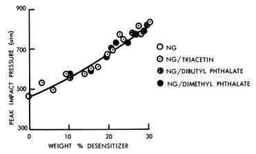
Figure 9. Impact pressure necessary to cause explosion (50% point) of nitroglycerin solutions when impacted from a height of 1 cm. with varying weights
