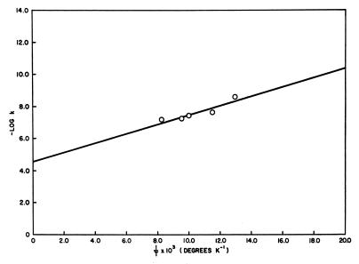
Figure 6. Arrhenius plot for O<sub>z</sub>F· formation
