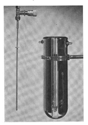
Figure 3. Special Dewar for holding sample during irradiation at -196°K.
