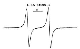
Figure 2. EPR of liquid OF<sub>2</sub> at 9.1 Gc ( $T = 77^{\circ}K$ .), after photolysis
