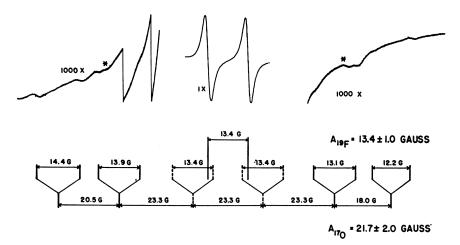
Figure 4. EPR of liquid OF<sub>2</sub>, 1% enrichment  $^{17}O$  (temperature = 77°K.), after photolysis
