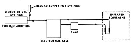
Figure 3. Arrangement for continuous water control and analysis by infrared
