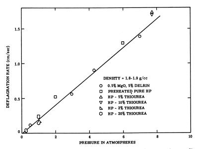
Rate of deflagration of hydrazine perchlorate with a small amount of fuel
