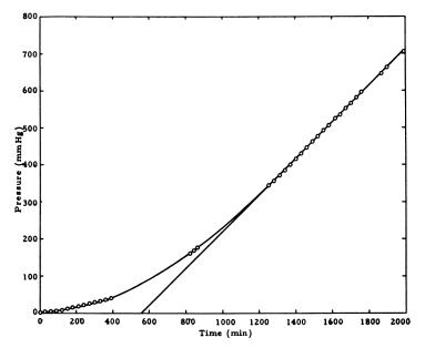
Figure 3. Pressure vs. time curve for hydrazinium perchlorate at  $140^{\circ}\mathrm{C}$ .
