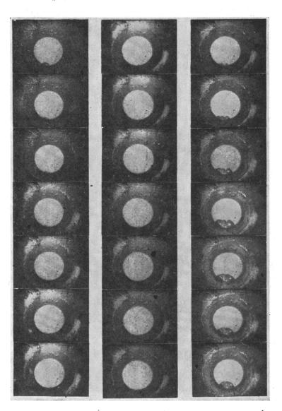
Figure 14. Photographic sequence showing impact compression and failure to explode because of increased sample size and corresponding decrease of air bubble volume; interframe time-222µsec. Sequence is top to bottom, left to right
