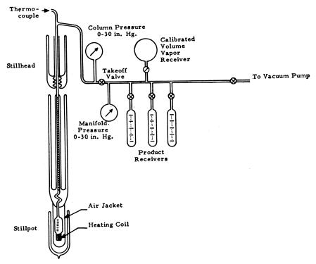
Figure 4. Schematic diagram of low temperature fractionation and gas chromatography apparatus
