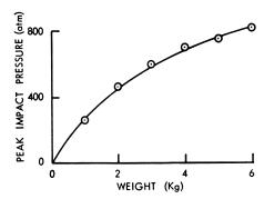
Figure 8. Peak pressure owing to impacting weight from a height of 1 cm.
