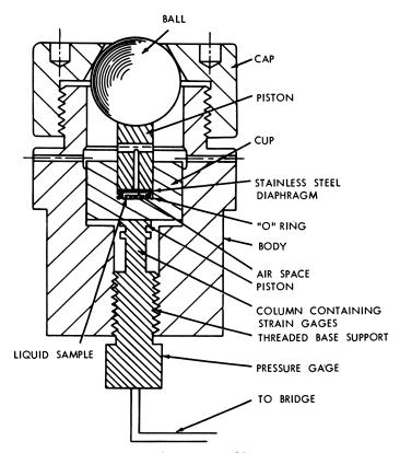
Figure 1. Details of sample cup assembly containing pressure gage
