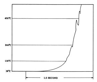
Figure 3. Tracing of thermocouple record of hydrazine perchlorate deflagration wave. Strand composition: 94.5% hydrazine perchlorate, 5% Delrin, 0.5% magnesium oxide; density: 1.85 grams/cc.; pressure: 0.5 atm.; deflagration rate: 0.09 cm./sec.
