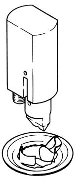
Figure 3. Effect of wedge breaking mechanism on rupture disk
