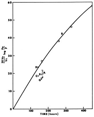
Figure 1. Reaction of NF: with NaOH solution at 100°C.
