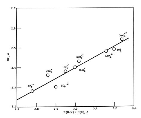
Figure 2. Correlation of thermochemical radius  $R_k$  with sum of bond distance R(B-X) and van der Waals radius R(X) in tetrahedral ions
