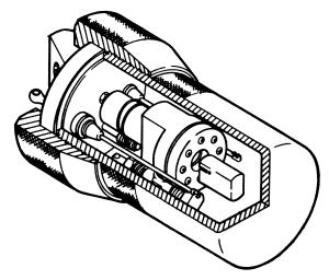
Figure 1. Nickel Parr combustion bomb with ampoule
