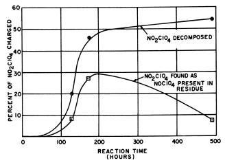
Figure 3. Decomposition of NO<sub>2</sub>ClO<sub>4</sub> at 65°C.
