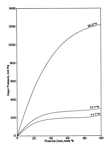
Figure 1. Vapor pressure of liquid ozone-fluorine mixtures
