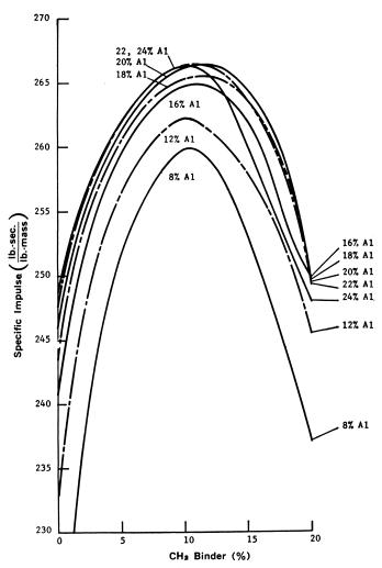
Figure 2. I., vs. percent binder at various Al levels for a  $+CH_{\bullet}$ \_+\_x/Al/AP propellant
