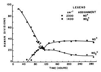
Figure 4. Raman analysis of decomposition of NO<sub>2</sub>ClO<sub>4</sub> at 65°C.
