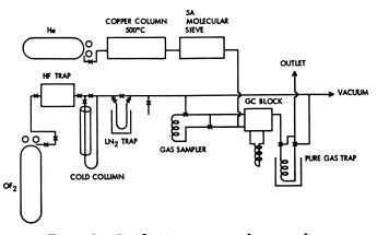
Figure 1. Purification system and vacuum line
