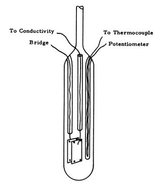
Figure 1. Conductivity cell
