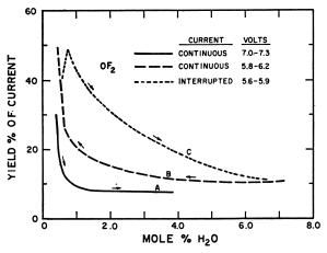
Figure 5. OF<sub>2</sub> yields at changing water concentration.  $KF \approx 1$  mole %, temperature =  $0^{\circ}-3^{\circ}C$ .
