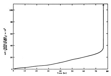
Figure 2. Pressure vs. time curve for hydrazinium diperchlorate at 120°C.
