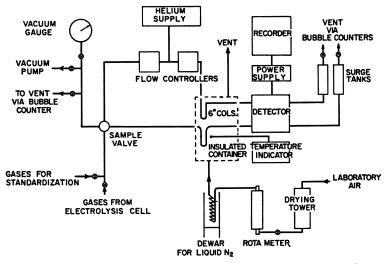
Figure 2. Low temperature programmed gas chromatograph
