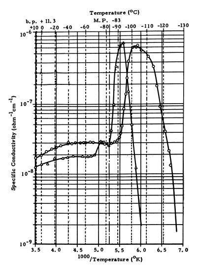
Figure 2. Conductivity of chlorine trifluoride as a function of temperature.  $\Delta$ —before low temperature fractionation; 0—after low temperature fractionation
