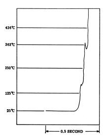
Figure 4. Tracing of thermocouple record of hydrazine perchlorate deflagration wave. Strand composition: 94.5% hydrazine perchlorate, 5% Delrin, 0.5% magnesium oxide; density: 1.24 grams/cc.; pressure: 1 atm.; deflagration rate: 0.30 cm./sec.
