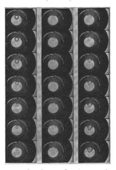
Figure 13. Photographic sequence showing impact compression and failure to explode because of high initial pressure; interframe time-111 µsec. Sequence is top to bottom, left to right
