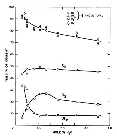
Figure 4. Yields at changing water concentration.  $KF \approx 1$  mole %, volts = 7.0–7.3, temperature =  $2^{\circ}$ - $3^{\circ}$ C.
