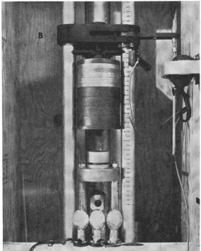
Figure 5. Apparatus for photographic studies, (A) showing location of camera, (B) showing location of posts, flashbulbs, and mirror below sample assembly; weights, release, and solenoid above
